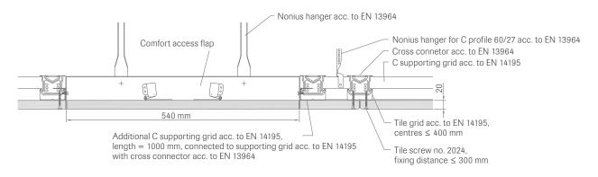
The access flap is inserted sideways into the opening and then aligned and fixed in place onto the C profiles using six screws no. 2024. Fine adjustment is possible in the area of the hinge mountings and the locking mechanism by unscrewing the Phillips screws and moving the unit vertically in the region of the slots. The corresponding RAW tile must be fitted onto the inspection hatch onsite. It must be bonded using adhesive no. 99/24.
