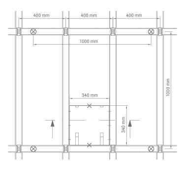
X = 2 additional nonius hangers acc. to EN 13964 + safety pin acc. to EN 13964 (2-fold)
