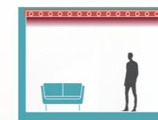
The heat radiates directly from the energy rails onto all the surfaces in the room.
