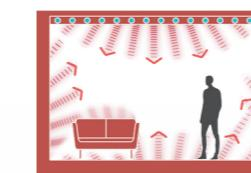
The water in the cool energy rails absorbs and dissipates the room's heat.
