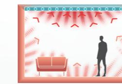
All the surfaces in the room are cooled to comfortably regulate body temperature without sweating.
