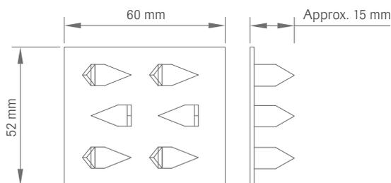
**6** Wall claw for 40/20 mm strong wall absorber, claw height 15 mm
