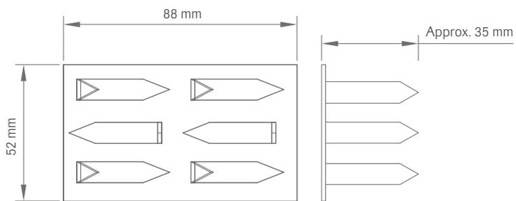
**6** Wall claw for 40 mm strong wall absorber, claw height 35 mm
