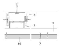
For execution without shadow gap (butt-jointed) the wall profile no. 51/22 can be omitted.
