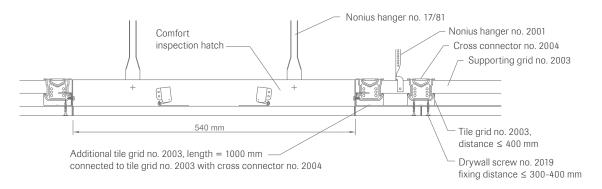
The inspection hatch is inserted correctly into the opening, aligned and bolted to the CD profiles with six screws. Fine adjustment is possible in the area of the hinge mountings and the locking mechanism by unscrewing the Phillips screws and moving the unit vertically in the region of the slots. The corresponding RAW tile must be fitted onto the inspection hatch onsite. It must be bonded using adhesive no. 9924.
