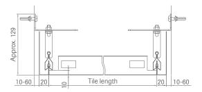
**Mounting distances:** wall anchor no. 75E: 500 mm hanger no. 1387E: 500 mm
