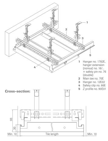
The hangers should always be placed at the crossing points of the supporting profile and the clip-in rail and should not be mounted further than 100 mm away from them. The maximum distance of the hangers is thus dependent on the length of the plates, but must not exceed a distance of 2000 mm.
