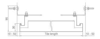
**Mounting distances:** wall anchor no. 75E: 500 mm Z profile no. 90E01: 500 mm
