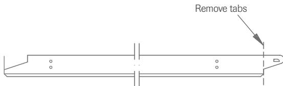
In the S 32 system, all panels can be folded down, apart from edge panels. For the easy disassembly of the edge panels, the "flaps" of the panels must be cut.
