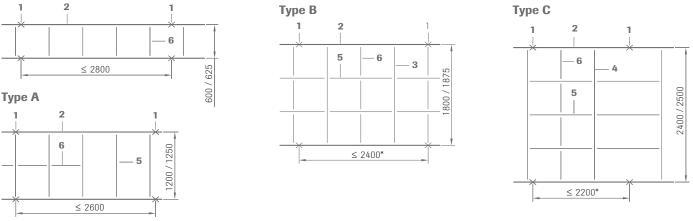
For additional overlay with mineral wool mats, the above mentioned spans must be reduced accordingly. Fittings on or in the ceiling, such as light fittings, sprinklers or air conditioning should always be suspended separately.
