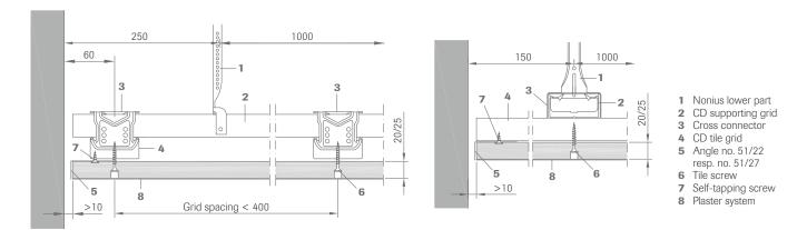
For fire protection, shadow gaps are not permitted. See section 3.1 of this installation guide.
