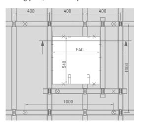
Additional supporting grid no. 2003, length = 1000 mm, attached to tile grid no. 2003 using cross connectors no. 2004
