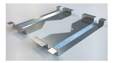
When installing downlights, mounting frame no. 8069/6 (two-part) is to be used. One mounting frame is required for each downlight. The frames must be placed with their edges on the CD profiles. Spacing between the frames depends on the diameter of the chosen downlight.
