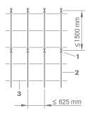
Module 625 x 625 mm, 610 x 610 mm or 600 x 600 mm
