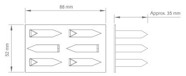
6 Wall claw for 40 mm strong wall absorber, claw height 35 mm
