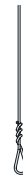
Pre-stressed wire \varnothing \geq 2.0 mm Fixing ends are bound at least 3 times
